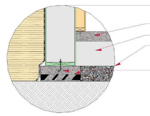
4" 20 MPa Concrete Floor 10" EPS Insulation 8-MIL Poly Vapour Barrier
