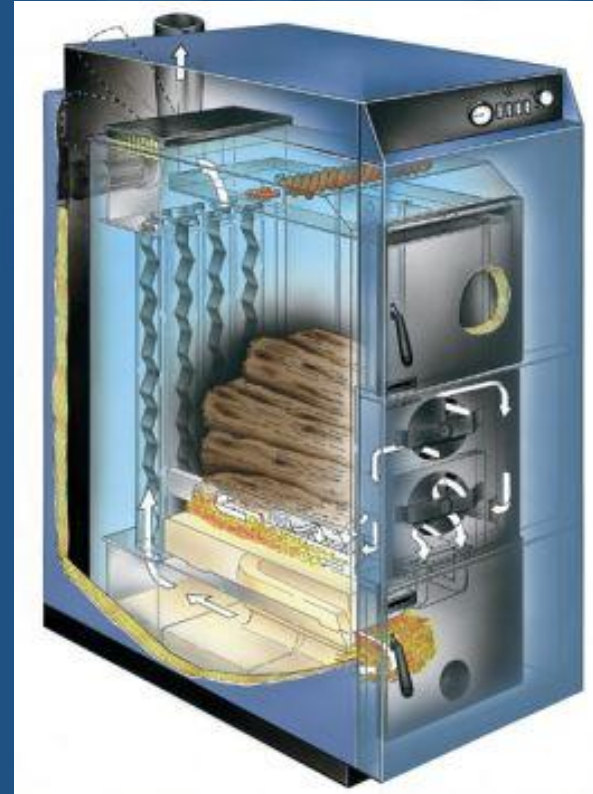
Cross-section of HS Tarm Solo Innova that burns cordwood
